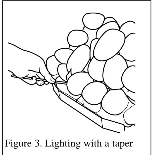
Figure 3. Lighting with a taper
